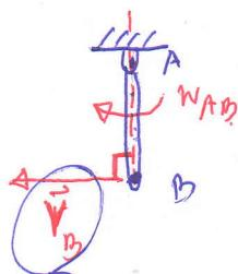
$$\begin{aligned}\vec{V}_B &= \vec{\omega}_{AB} \times \vec{r}_{B/A} \\ &= -2.7 \vec{k} \times [-0.125 \vec{j}] \\ \vec{V}_B &= -0.3375 \vec{i}\end{aligned}$$
