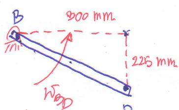
$$\begin{aligned}\vec{V}_{GP} &= \vec{V}_T + \vec{V}_R \\ \vec{V}_D &= [\vec{V}_D]_{\text{Translation}} + [\vec{V}_D]_{\text{Rotation about B}} \\ \vec{V}_D &= \vec{V}_B + \vec{V}_{D/B} \\ \vec{V}_D &= \vec{V}_B + \vec{\omega}_{BD} \times \vec{r}_{D/B}\end{aligned}$$
