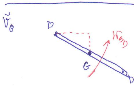
$$\vec{V}_G = [\vec{V}_B]_T \text{ with } B + [\vec{V}_G]_R \text{ about } B$$
